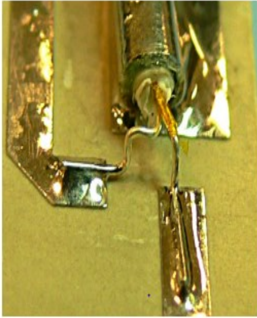
Fig. 13. element of the inner conductor coaxial coupler connected to the microstrip. A resin with unknown SEY is used to prevent discharges.
